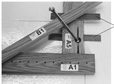
Both washers for each screw should be under the head of the screw, and not between the wood parts.
