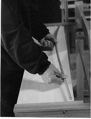
Stop Rods are used to keep items from sliding off tilted Work Boards. To install, insert one end of Stop Bar into hole in Board Side. Bend Stop Rod as shown to install other end of Stop Rod in corresponding hole in opposite Board Side
