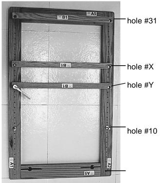
Position Stationary Slides over Legs of Left Hand End Frame Assembly as shown. The Stationary Slides have (2) counterboared holes. As these holes are offset, position all Stationary Slides with offset holes down.
