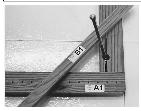
Both washers for each screw should be under the head of the screw, and not between the wood parts.
