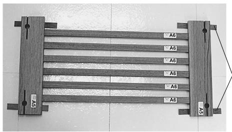
Place (4) A7 End Frame Gauges under blocks of one of the (2) Block and Slat Sub-Assemblies.
