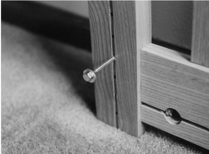
Insert (2) 1/4" X 3" screws with (2) washers under their heads into leg holes as shown.
