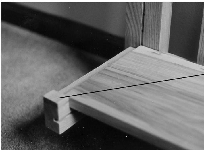
Drop Carrier Board onto Stub Rails.
