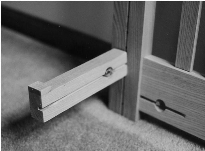
Slide Stub Rails onto screws.
